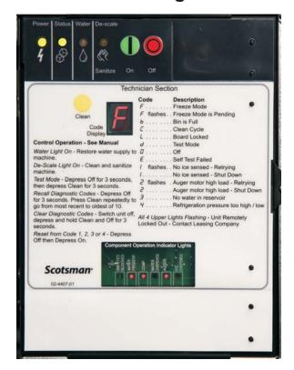
At the beginning of any restart the controller will display a blinking F.
