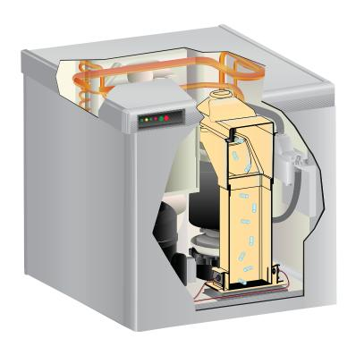
The control system checks for operation by using the photo-electric eyes to detect ice as it is made.
