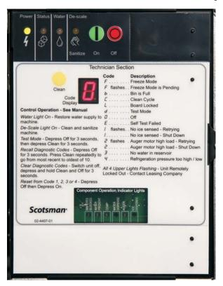
When power is supplied, the four lights at the top and the display indicator will blink on and off one time. Then the Power light will be on and a  $\mathfrak{D}$  is displayed.
