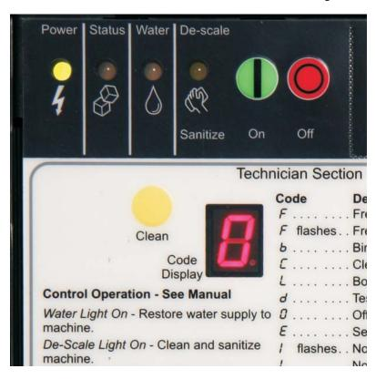
The control can be put into a Test Cycle, where it switches all the loads on and off in a logical sequence. This allows the technician to confirm controller operation of all parts.
